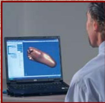
Once the scan is complete the resulting data is converted into an accurate 3D model and can be modified to accommodate the needs of the patient. This modification can be done by either the clinician or by Acor's trained clinical staff using the Omega<sup>®</sup> Tracer<sup>®</sup> CAD system. A complete array of foot orthotics are available.
