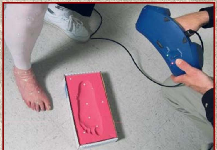
... and here the bottom of the foot is scanned, in the negative depression of the foam mold. Carefully placed reflectors maintain the relative positioning.
