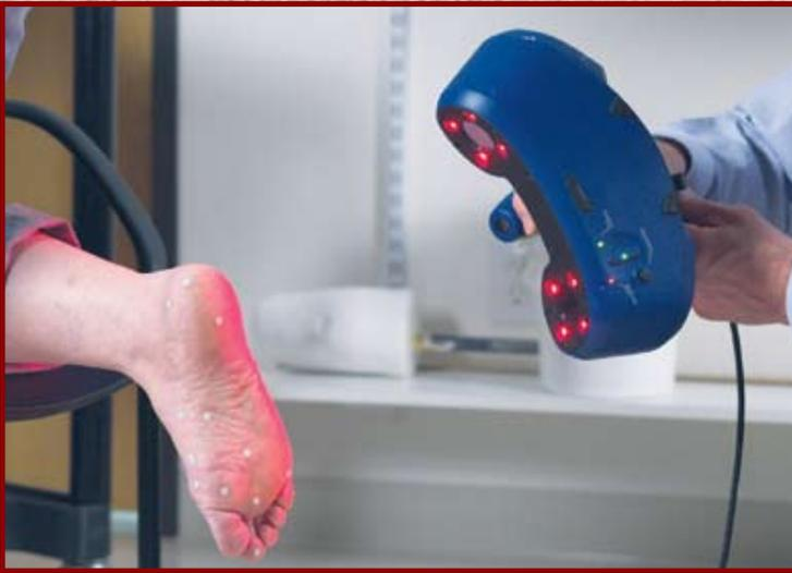
... and here the bottom of the foot is scanned directly.
