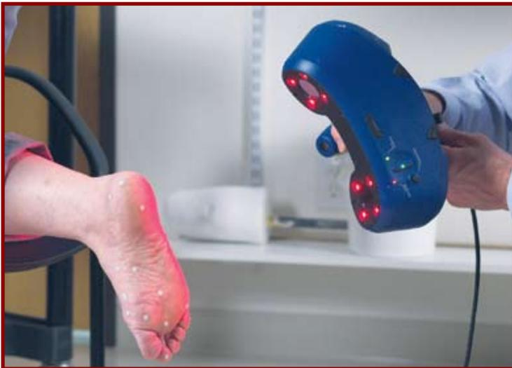
... and here the bottom of the foot is scanned directly.
