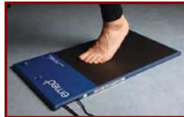
The TrueContour™ system comprises shape and pressure measurement devices (pictured above), operated by an easy-to-use graphical user interface through which the practitioner gathers, and then transmits, the patient data to Acor's central fabrication facility.
